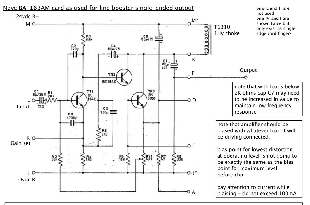
GAIN: this amplifier has an inherent gain of 11dB to pin F. The gain can be increased by taking pin K to ground (pin J) through an R and a C = the C assures gain is only increased for audio (not dc) and the R sets the AC gain R=1K2 and C=100uF will increase gain to 16dB
